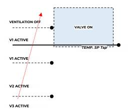
The shaded area represents the temperature range defined by the "heating control differential ON" parameter in case of increasing temperature.
